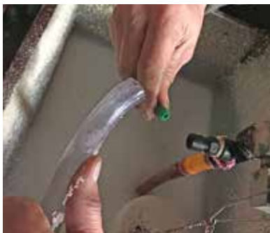
Check the metering tip for any blockage
