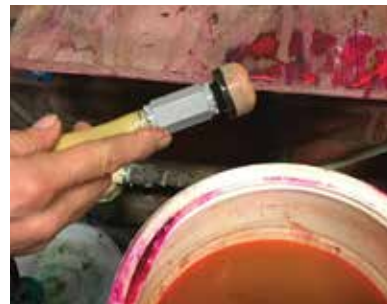
Check the holding tank hose filter
