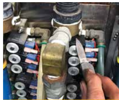
Check the coil with a piece of metal
